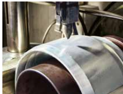
2. Ferrule marking for full traceability
